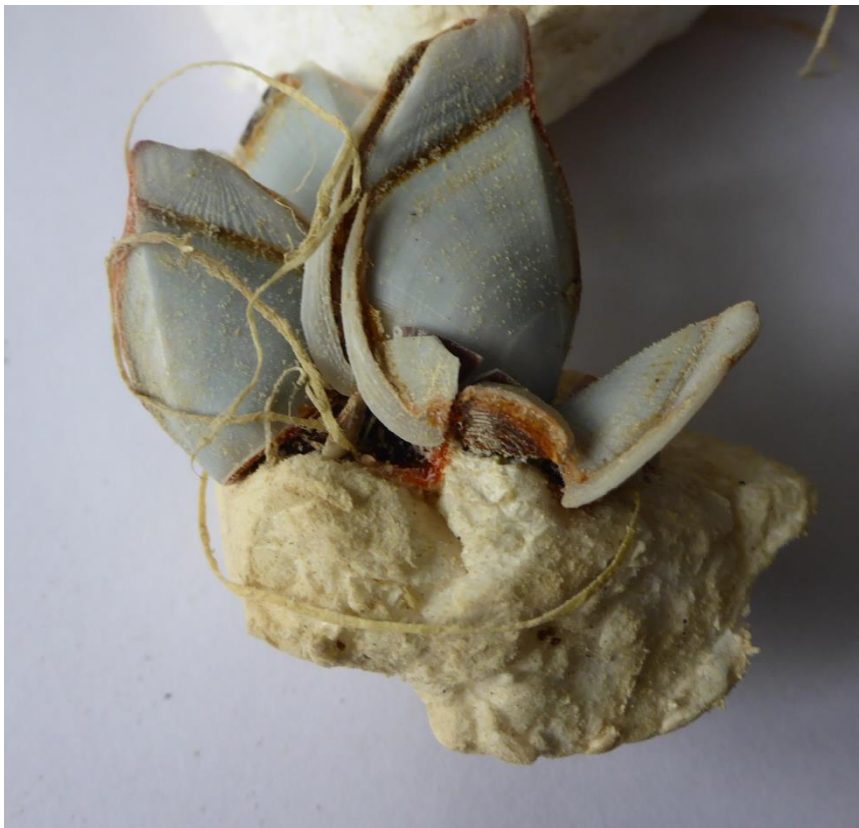
Figure 19 : Photo-oxidised EPS fragment with a yellowed surface and forming a yellow powder (Source: Cedre)
