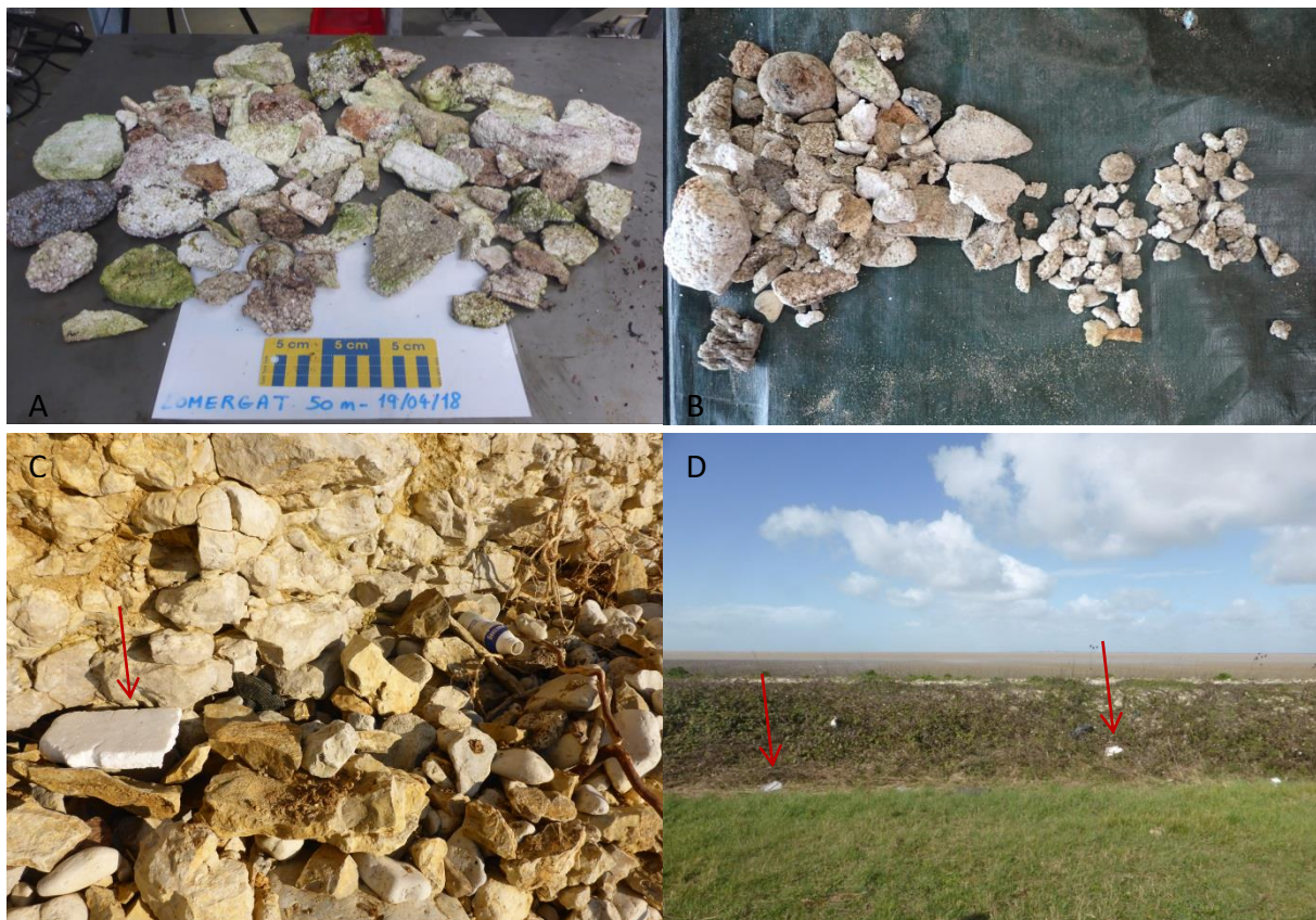
Figure 17: EPS/XPS non identifiable fragments found on the French coastline (source: Cedre). A and B: fragments collected in the Bay of Brest, C: fragment observed on the Oléron island coastline (indicated by the red arrow), D: Marine EPS fragments blown inland, behind the beach by the wind in Marsilly (indicated by red arrows)
