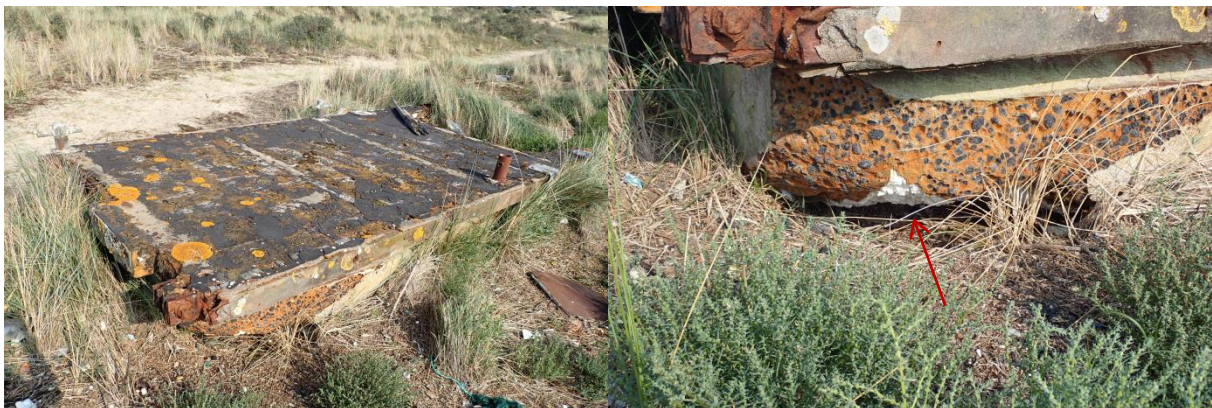
Figure 36 : Floating pontoon partly made of EPS (as indicated by the red arrow), observed on the French coastline (source: Cedre).
