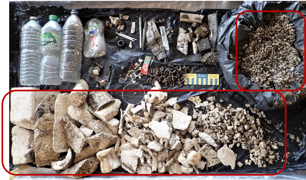
Figure 30: Multisize EPS collected in a floating siphon in Brest rainwater system (surrounded in red) (source: Cedre)
